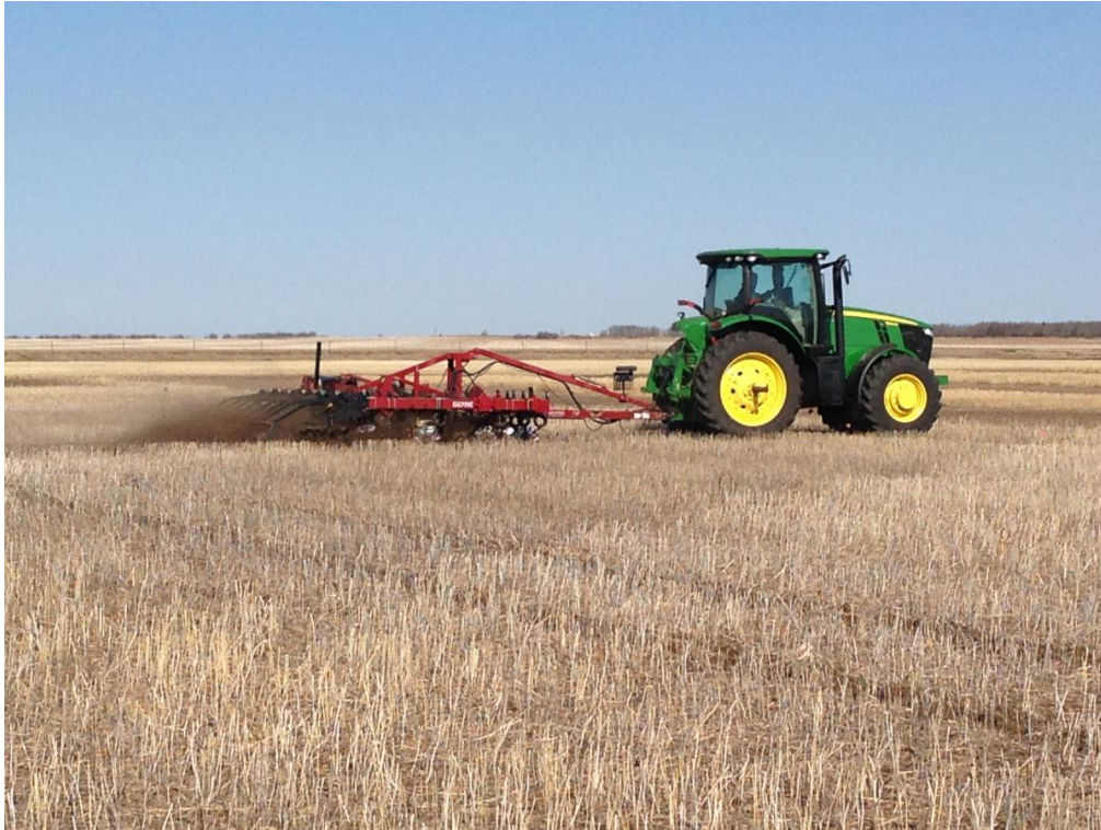
Figure A.1. Vertical tillage implement applying tillage treatments in demonstration plots May 13, 2014
